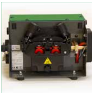
RWF 2 – compact feeder for MIG with four-roll wire feed system and electronic tacho control of wire feed speed.
